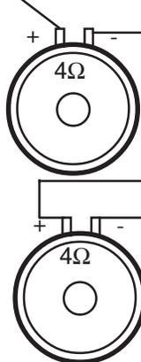
Connection of two subwoofers with 4 ohm voice coils in series
