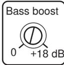
This function is used to compensate for the bass box function and to adjust for your own taste of bass. Set level control at 0 dB if you want it to be inoperative.
