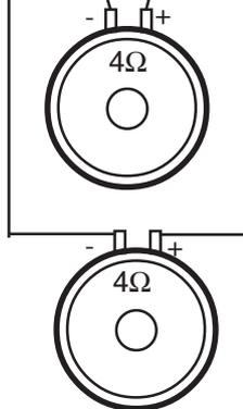
Connection of two subwoofers with 4 ohm single voice coil
