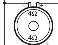
Dual voice coil subwoofer connected in parallel in bridge mode.
