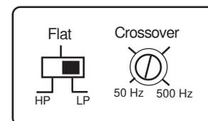
Set the switch in position LP to activate the filter.
