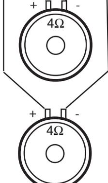
Single voice coil subwoofer connected in bridge mode.
