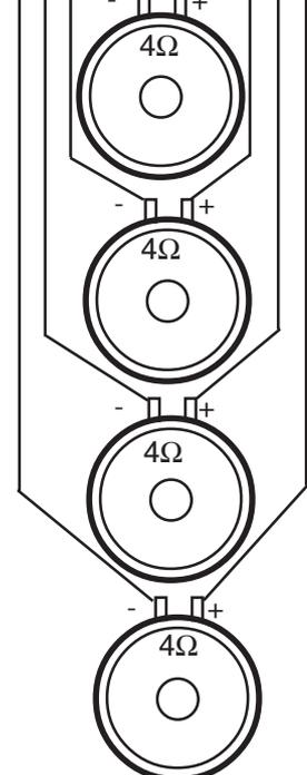
Connection of four subwoofers with 4 ohm single voice coil
