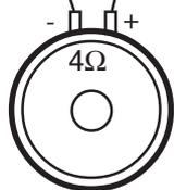
Connection of a subwoofer with 4 ohm single voice coil
