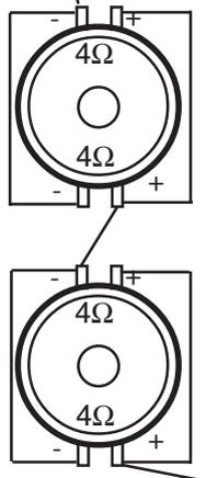
Connection of two subwoofers with 4 ohm dual voice coils in parallel and then in series to the amplifier with a resulting impedance of 4 ohms.
