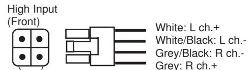
Hi level input plug on amp for CH L/R.
