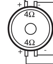
Connection of a 4 ohm dual voice coil subwoofer with the voice coils in series.
