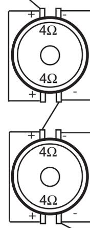
Connection of two subwoofers with 4 ohm dual voice coils in parallel and then in series to the amplifier gives a resulting impedance of 4 ohm.
