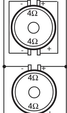
Connection of two subwoofers with 4 ohm dual voice coils
