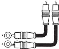
**X-D40** has dual inputs Front R/L & Rear R/L. Depending on your chosen configuration you can use either two separate RCA cable, or a single RCA cable together with an Y-split to connect both inputs.
