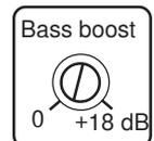
This function is used to compensate for the bass box function and to adjust for your own taste of bass. Set level control at 0 dB if you want it to be inoperative.
