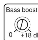
This function is used to compensate for the bass box function and to adjust for your own taste of bass. Set level control at 0 dB if you want it to be inoperative.
