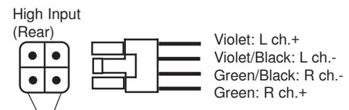
Hi level input plug on amp for CH L/R.
