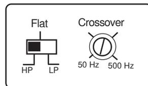
Set the switch in position HP to activate the filter.
