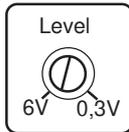
Play a CD, make sure all bass or treble settings or equalizer are flat, and turn the volume of the radio up until you just start to hear distortion. Turn the volume control down just a bit. On the amplifier increase the input level control ( clockwise or to the right ) until you just start to hear distortion, then back the level control just a bit. Now your radio and amplifier levels are matched.
