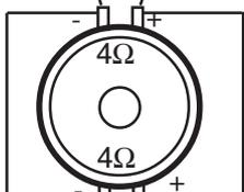
Connection of a subwoofer with 4 ohm dual voice coils
